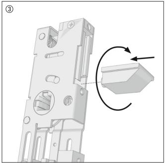
To change the backset, place the spacer strips onto the lock case. For a centre distance of 72 mm, first shorten the spacer strips at the predetermined breaking point.
