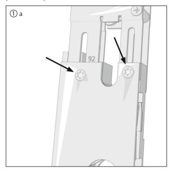
Lift the lever on the rear face with a screwdriver. Now push the lock case together until you feel the stop. Then push the lever again into its original position.
